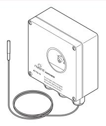
nVent RAYCHEM AT-TS thermostats provide temperature control in safe area. The temperature set point can be checked through a window in the lid. LED's are providing an indication when cables are energized (Heating ON) or when the temperature sensor is defect (sensor break or sensor short-circuit).
