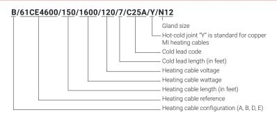
In the above heating cable catalog number, the length of the heated section and the cold lead are in feet. For metric lengths, the heating cable catalog number would include a suffix "M" after the length, as shown below. A LSZH jacket on the heated section and a LSZH jacket on the cold lead have also been included in the following: B/61RE4600-RD/45.7M/1600/120/2.1M/R25A/Y/N12
