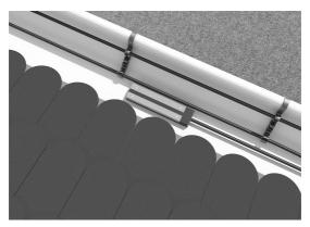
Moisture sensor positioned in the gutter
