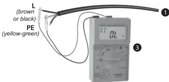
Insulation's resistance measurement
