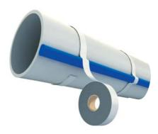
For plastic pipelines, fix additionally selfadhesive aluminum foil along the heating cable to improve the temperature distribution on the surface of the pipeline. Additionally, the aluminum foil will secure the cable from being pulled into the thermal insulation.
