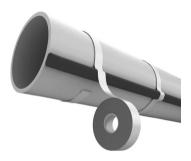
For plastic pipelines, install self-adhesive aluminium foil on the pipe before fixing the heating cable. This will improve the temperature distribution on the surface of the pipeline,
