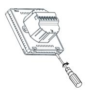
Connect the electric wires and the sensor, then install the controller in the connection box and fix the controller display to complete the installation.
