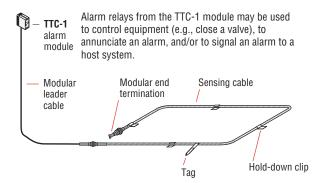
Sensing cable can be positioned to provide complete leak detection coverage of pumps, boilers, and other equipment.
