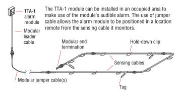
**Note:** A TraceTek alarm system can include several lengths of sensing cable. However, for large and/or separate areas, consider a TraceTek locating system.
