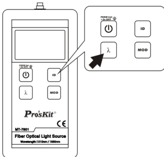
After pressing “ $\lambda$ ” button, you can select the required output wavelengths. Details refer to the parameters table.
