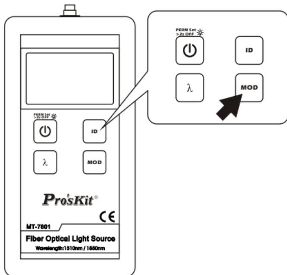
After pressing “ MOD ” button, you can load a confirmed carrier frequency in the current output laser.
