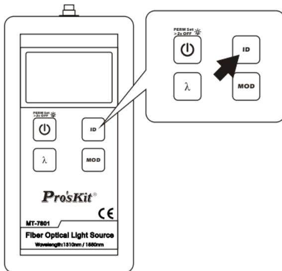
Press “ ID ” Button, it start the wavelength recognition function, and the upper left of the display screen shows 'Id'. When connect with the power meter supporting wavelength recognition function, it can show the current output wavelength of light source, and switch to measure the wavelength automatically.
