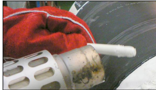
Heat the tip of the PP-Meltstick with the hot air tool.
