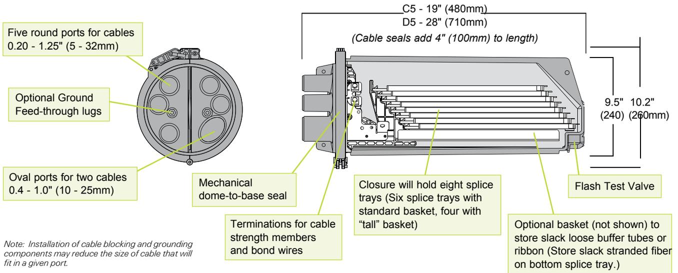
*Note: Installation of cable blocking and grounding components may reduce the size of cable that will fit in a given port.*
